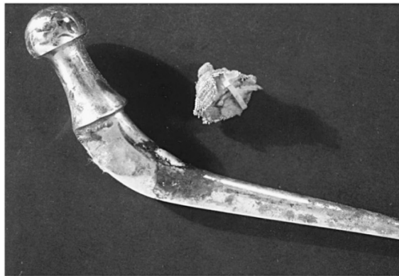
Figure 2. Failure of stainless steel implant due to corrosion [11].
