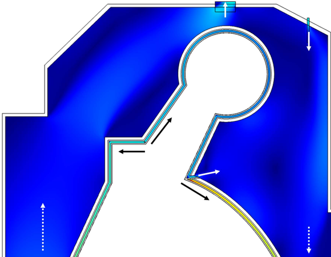
Figure 4 Inlet-outlet configuration in ARC vessel and tank. The auxiliary inlet has been moved from the initial configuration defined in [2].
