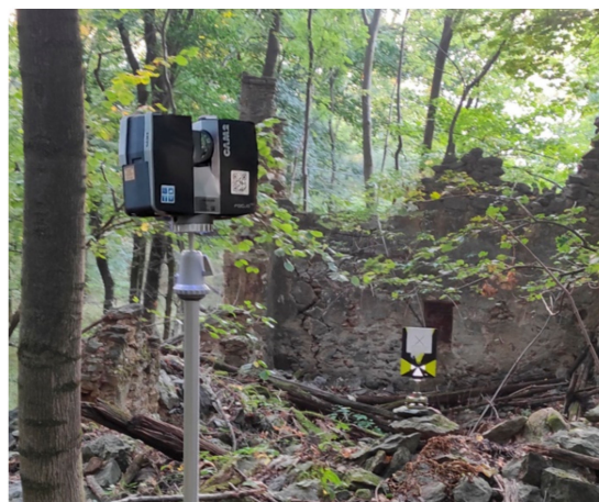
Figure 6. Faro Focus 3D X130 Terrestrial Laser Scanner device used for the detailed digitalization of the building and its environment. On the left, the laser scanner is shown during data collection and on the right the equipment in detail.
