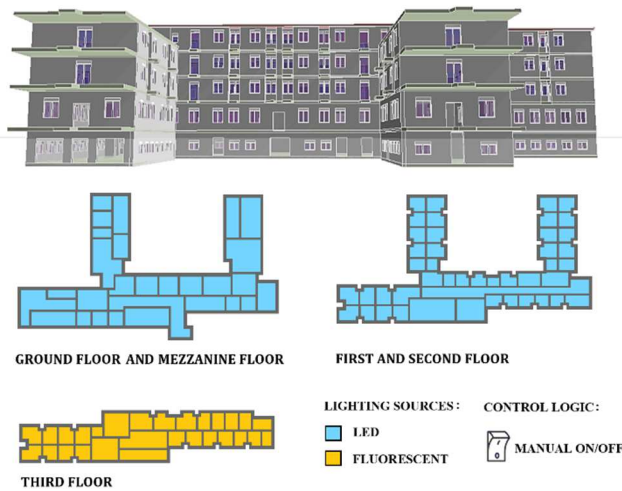
Fig. 4. The Brancaccio retirement home with the actual lighting system
