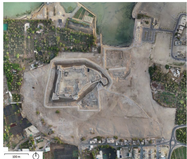
Figure 1. Orthoimage produced from unmanned aerial vehicle (UAV) photogrammetry captured at 100m flight height. It shows the forts, archaeological tell and surrounding agricultural lands, World Heritage Site property of Qal'at al-Bahrain - Ancient Harbour and Capital of Dilmun. Source: authors data processing.
