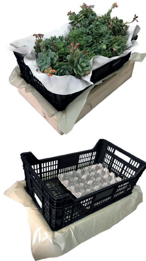
Figure 22 | The constructed Blue-Green Roof Module prototype. Source: Caterina Dadati and Marco D’Amico.
