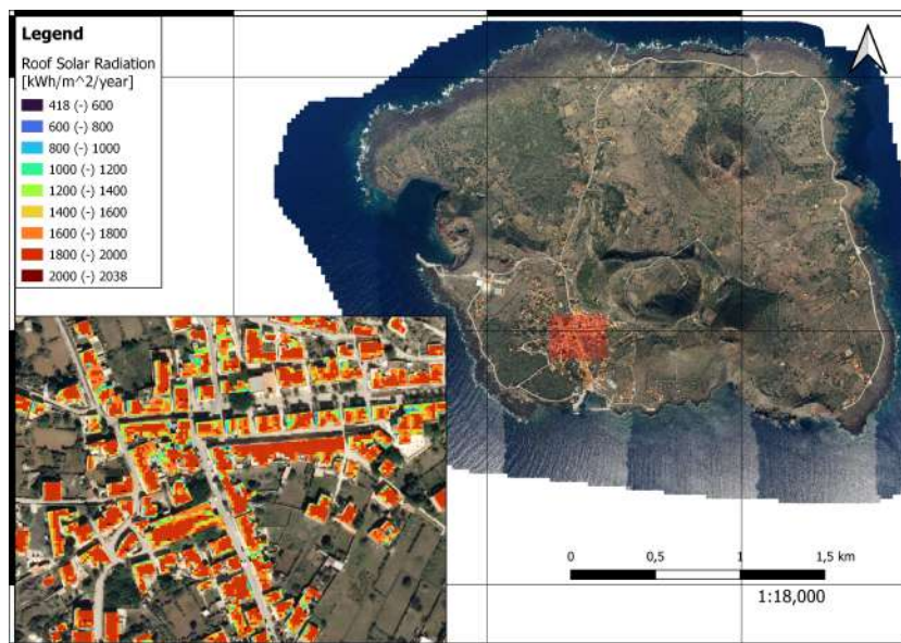
Figure 21. Solar radiation on Linosa roofs.
