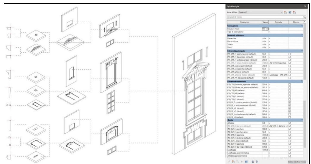
Figure 3. Nesting procedures for the building component collection: local models and geometric parameterization. Image by the authors.
