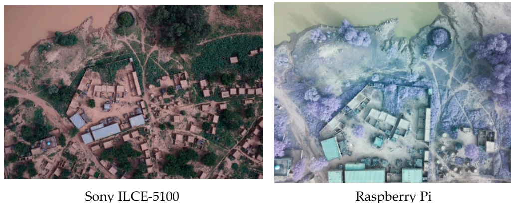
Figure 4. Sample pictures of the same area acquired by Sony-ILCE-5100 and Raspberry Pi. The SONY picture ( 6000 \times 3000 pixels) has a 3.9 cm/pixel resolution and is in RGB. The Raspberry picture ( 2592 \times 1933 pixels) has a 6.1 cm/pixel resolution and is visualized in red-green-NIR false color composition.
