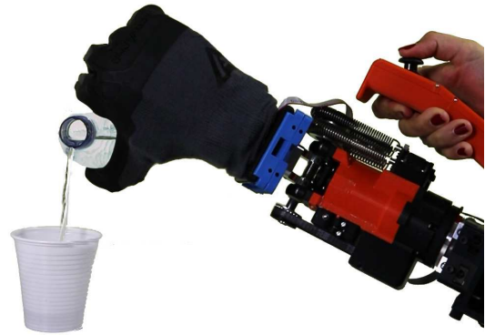
Fig. 1. The two DOFs adaptive under-actuated wrist pouring water.
