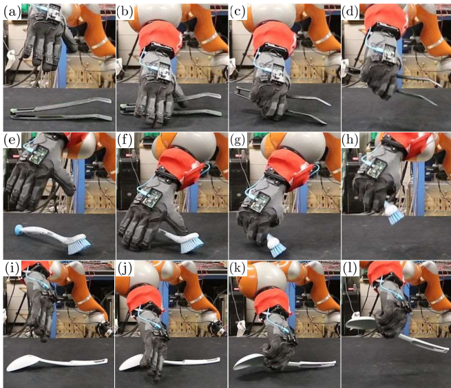
Fig. 9. Photosequences of grasps produced by the proposed architecture during validation: panels (a-d) present a pinch grasp of object 7, panels (e-h) a pinch-left grasp of object 8, and panels (i-l) a pinch-right grasp of object 9. Panel (a) shows the hand initial configuration. The contact is established in panel (b) through interaction with the environment, which also guides the hand towards the grasping achieved in panel (c). In (d) the object is firmly lifted.
