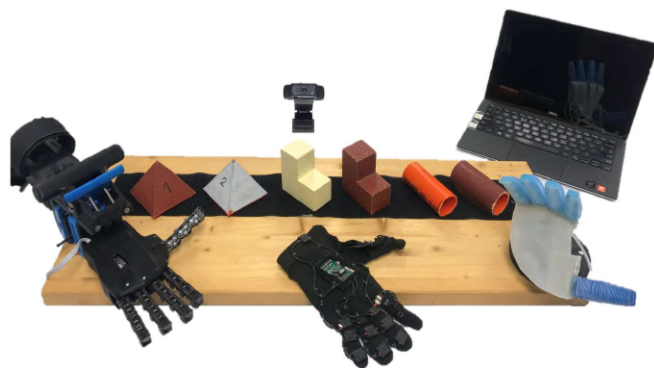
Fig. 5. Experimental Setup used in this paper. Two soft robotic hands (namely RBO Hand and Pisa/IIT SoftHand) were used to grasp six objects with different shape and surface roughness. A camera was used to record the whole experimental execution. Accelerations of the fingers were recorded through a custom glove endowed with 16 IMUs.
