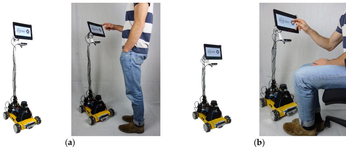
Figure 5. Final prototype of the mobile assistive robot in two different working configurations: (a) Deployed configuration for standing usage, HMI height = 1.1 m, mechanism tilting angle = 0^\circ , (b) Retracted end angled configuration for better-seated usage, HMI height = 0.80 m, mechanism tilting angle = 20^\circ .
