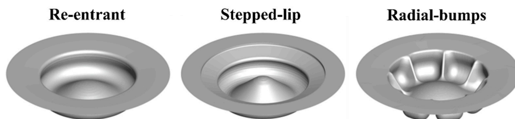
Figure 1. Isometric view of the piston bowl geometries: (left) re-entrant; (middle) stepped-lip; (right) radial-bumps.
