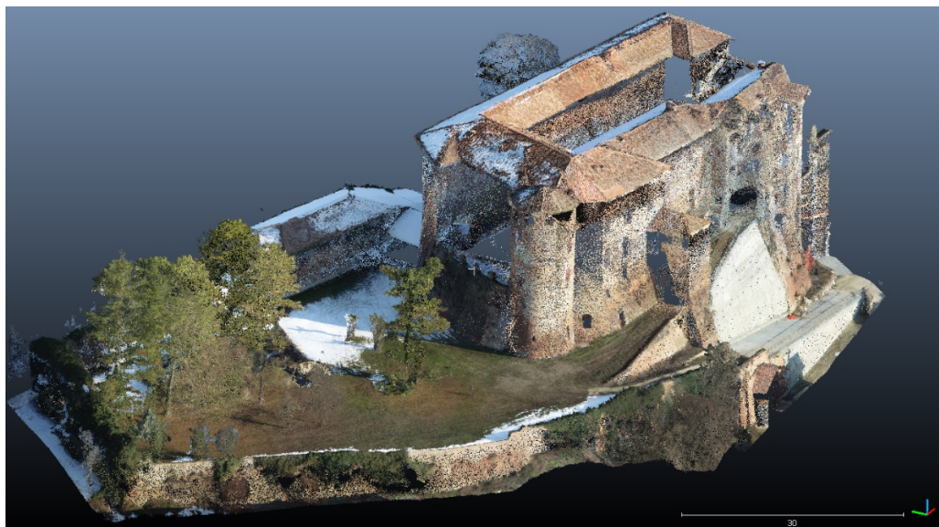
Figure 5. Zenmuse L1 point clouds data related to the castle and the near surroundings within the perimeter walls.
