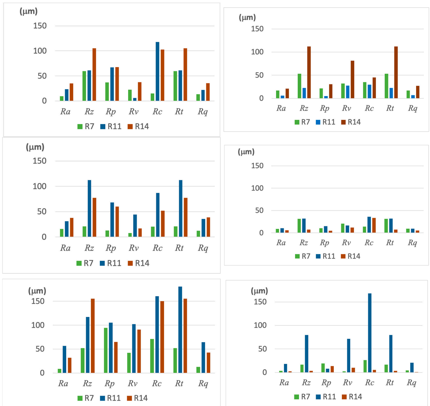
Figure 7. Roughness difference after and before wear test for Ti-Dia (left) and Ni-Dia (right) coatings for different measuring points: left (top), right (center) and top (bottom) measurements.
