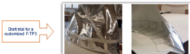
Figure 30 EFESTO 1:2 Ground demonstrator – simulacra of the F-TPS.
