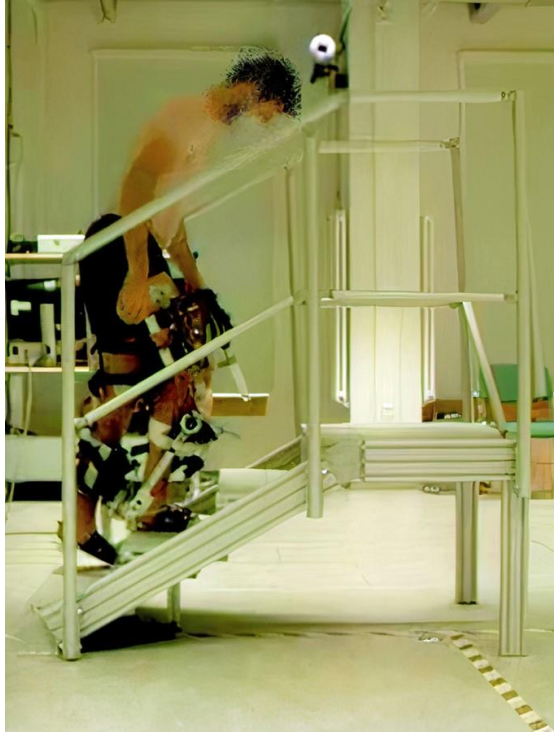
Figure 2: Trial of a stair ascent with the supporting exoskeleton on both legs.
