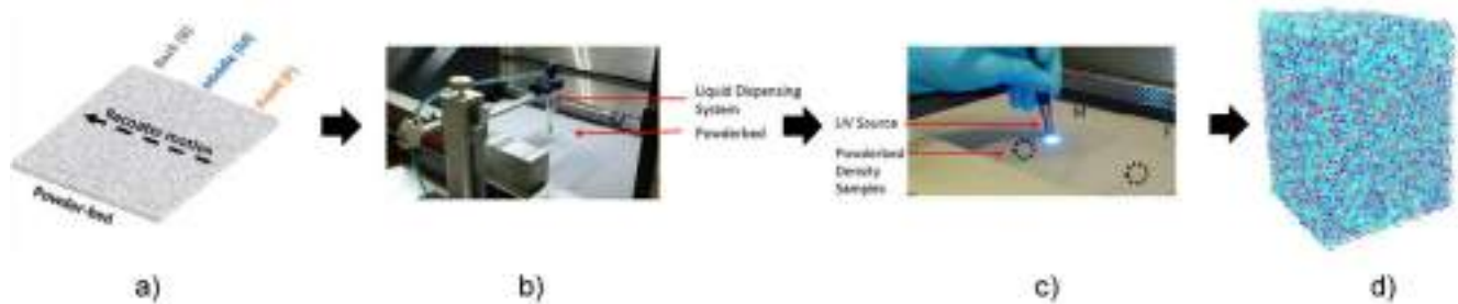
Figure 20. Powder bed density measured after the a) spreading, b) dispersion of UV-curable solution, c) curing the solution and d) perform nano-CT and postprocess the data. Modified after Ali et al. (2018).
