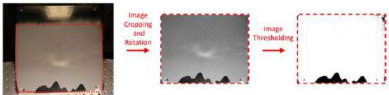
Figure 17. Determination of the percentage of layer coverage by using image analysis Snow et al. (2019).
