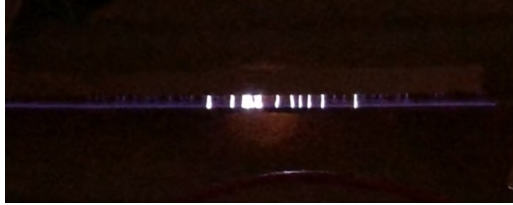
Figure 4: Photography of the CD between the exposed electrodes of actuator A and B for tested case 1.
