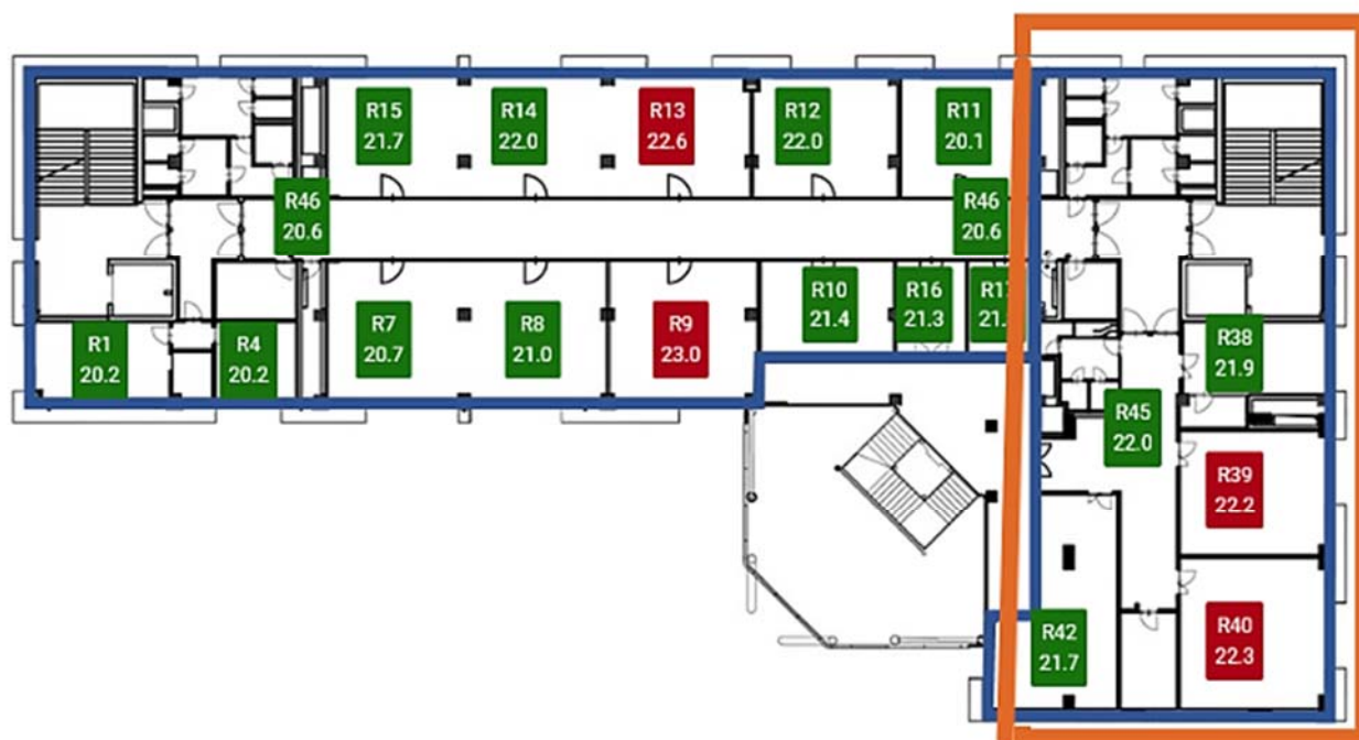
Figure 2. Energy Center layout. The layout is shared by all the considered floors. Green boxes indicate that the room set-point has been reached, red indicates a thermal discomfort situation with respect to the room set-point.
