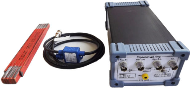
Fig. 7: Rogowski coils with the corresponding electronic integrator.
