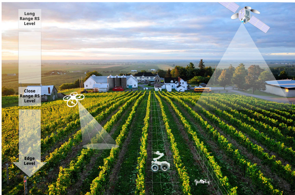
Figure 1.2: Data ecosystem of a precision agriculture application. Long and close-range RS acquired data can be processed by ML algorithms to extrapolate valuable information for the overall process. Subsequently, machines at the edge layer, guided by information of previous levels, are driven by similar ML techniques, optimized to run locally and efficiently onboard the machines for navigation, decision-making, and task execution.
