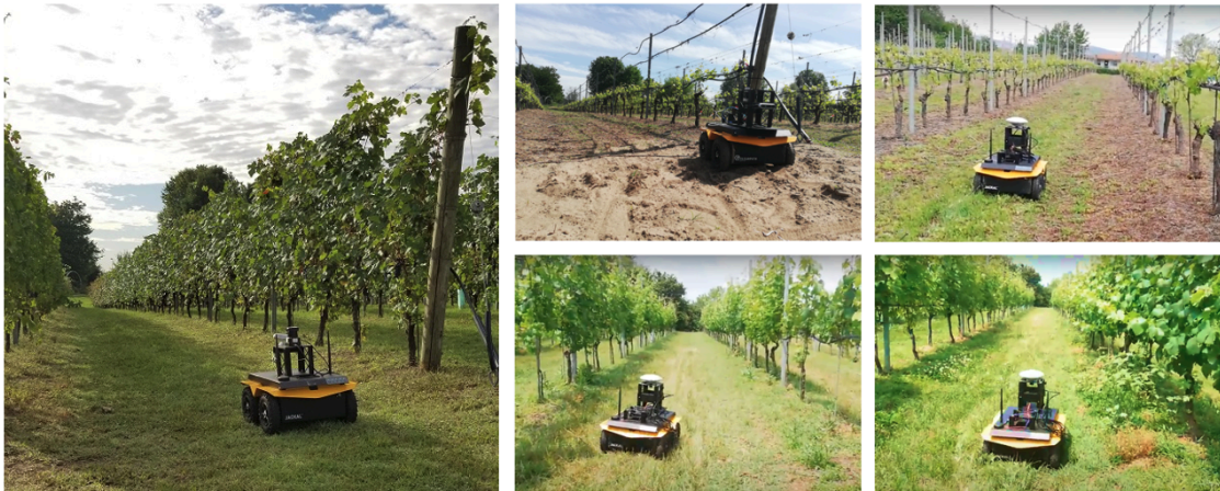
Figure 7.1: Field tests with the Jackal platform in different seasonal periods of the same crop. Lush vegetation and thick canopies significantly reduce the GPS accuracy, affecting its reliability and consequently the overall navigation pipeline. Nevertheless, our proposed segmentation-based algorithm exploits semantic segmentation properties to provide a proportional controller that drives the robotic platform along the whole row.
