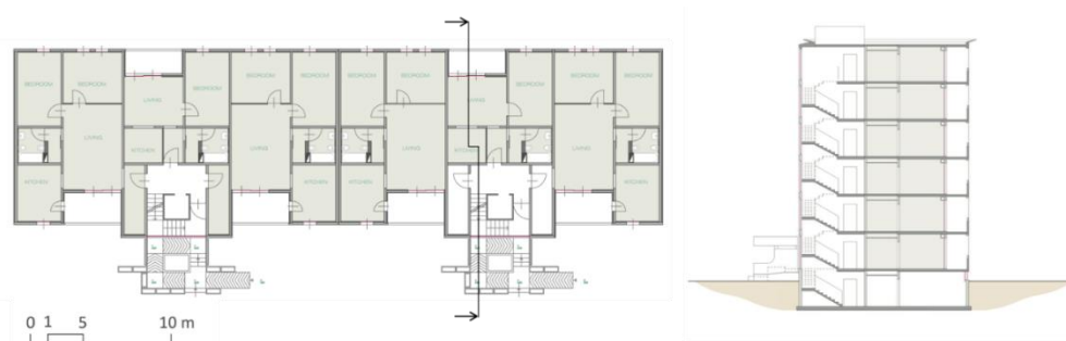
Figure 3. Architectural drawing of the plan (on the left) and section (on the right) of the Reference Building.
