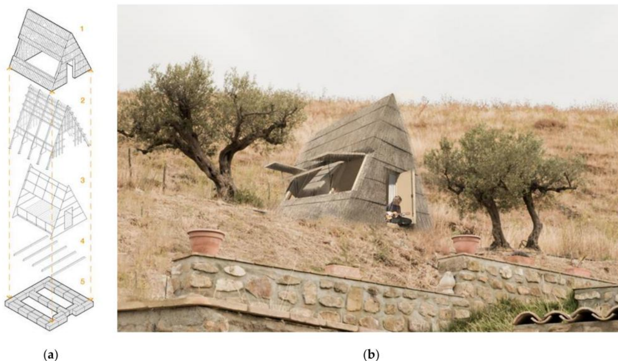
Figure 6. (a) Exploded axonometry of the layers: (1) Water reed layer; (2) Triangular frame structure; (3) Wooden layer; (4) Base of the triangular structure; (5) Base of gabions filled with rocks. (b) Rendering of the Pagliaru Novu inside the project area. With the addition of the word Novu —“new” in the Sicilian dialect—we aimed to summarize the three innovation concepts we have worked on and specify that the design presented is an evolution of the classic pagliaru .
