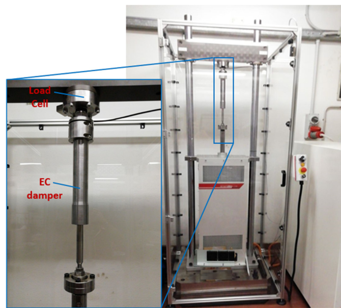
Figure 5. The Laboratory test rig used to experimentally validate the EC damper FE model prototype.
