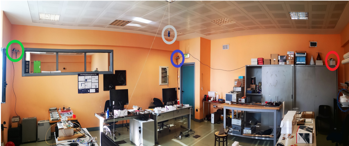
Figure 4.1: Indoor laboratory measurement setup. In green, red, blue and gray are highlighted respectively the three Sensors and reference Tag positions.
