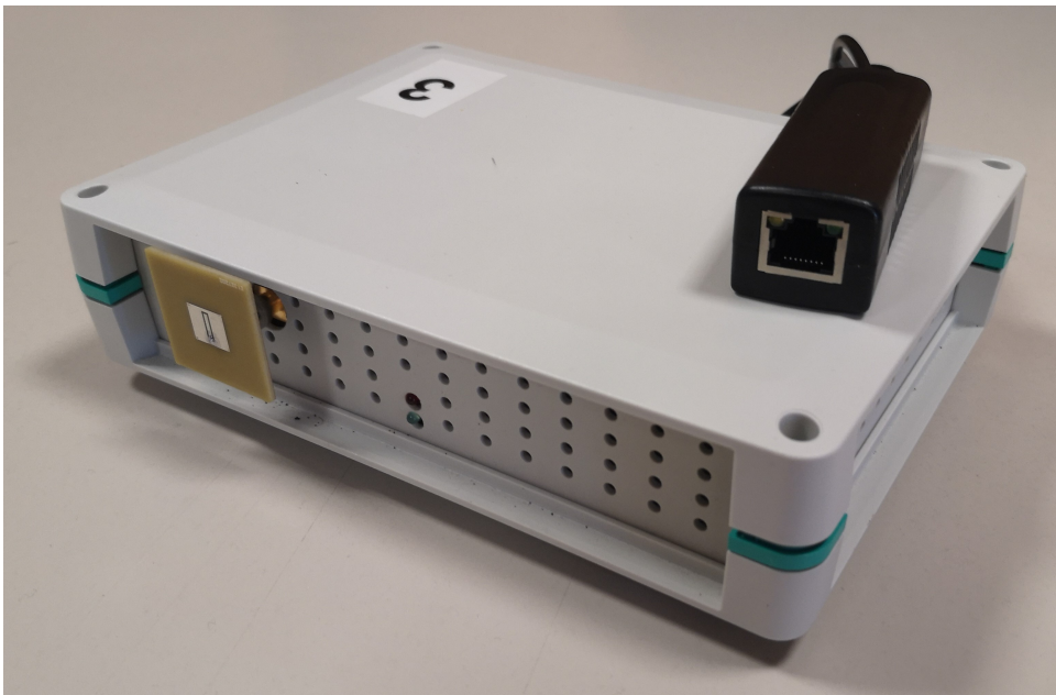
Figure 2.42: Final aspect of the Sensor board enclosed in the box.
