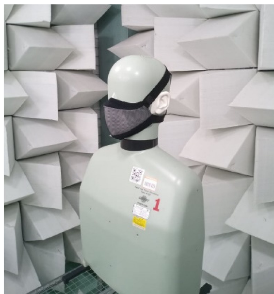
Figure 4. Mask S on the Head and Torso Simulator in the anechoic chamber of Politecnico di Torino.
