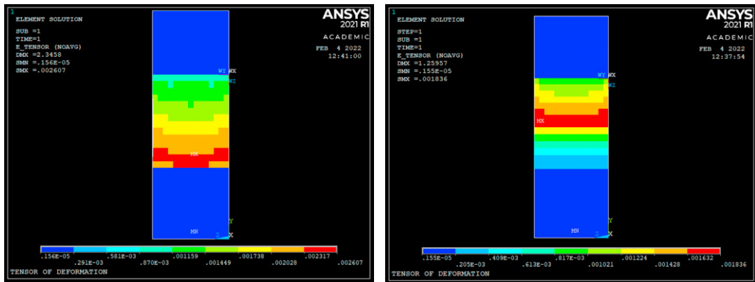
Fig. 3. Strain tensor norm contour for the two samples after static analysis under the alternated load (100 N) component.
