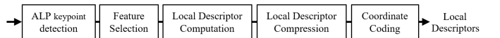
Fig. 2. Normative process for extracting local descriptors from a single image in the MPEG CDVS standard.
