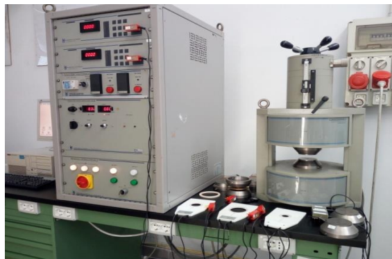
Fig. 7. The hysteresisgraph: view of the measurement system.
