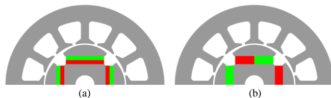
Fig. 2. Variable flux PM synchronous machine configurations (red: low coercive force magnet, green: high coercive force magnet): a) series magnet; b) parallel magnet. (adopted from [16])
