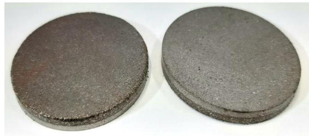
Fig. 5. Double-layer samples formed by bonded and hybrid magnets (on the left hybrid 70% and on the right hybrid 40%).
