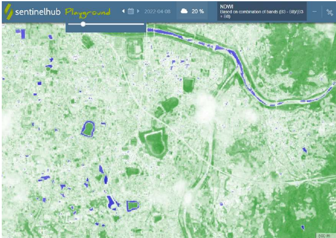
Fig. 29 – Sentinel Hub map of NDWI (based on combination of bands (B3 - B8)/(B3 + B8), date of the map 8 April 2022. The Normalized Difference Water Index (NDWI) is a remote sensing derived index estimating the leaf water content at canopy level.
