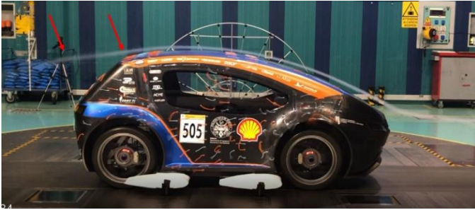
Figure 31 Standard configuration, JUNO's smoke wind tunnel test
