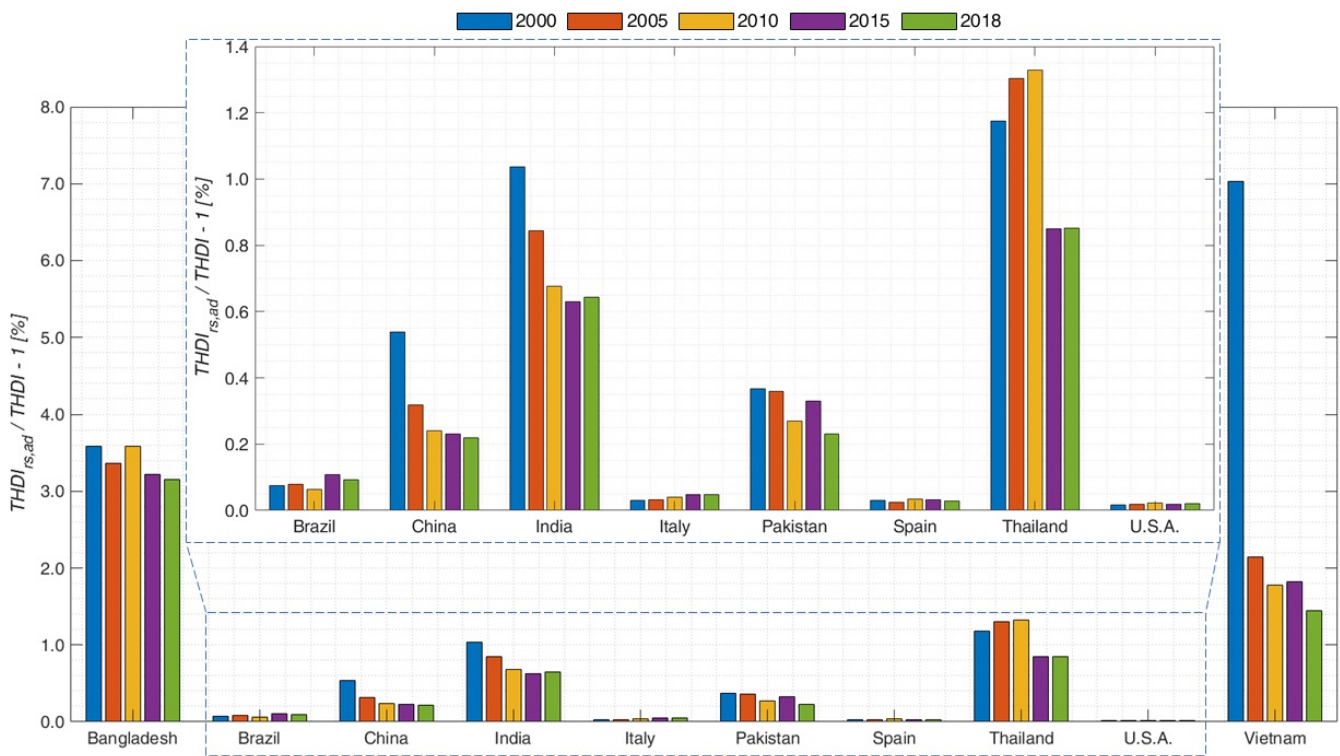
Figure 4. Yearly annual variation of the sustainability indicator THDI using Equation (11) to compare the current situation (50% of total rice straw burned on field) with anaerobic digestion of the same amount of rice straw to obtain biomethane using k = 0.70 in Equation (1).
