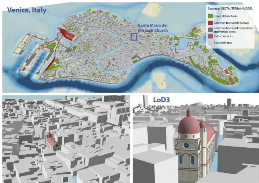
Figure 8. LoDs visualisation of St. Maria dei Miracoli, GIS project of the case study visualised in ESRI ArcGIS. QGIS could be used too
