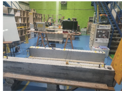
Fig. 1. (a) Schematic presentation of the beam with the central bar; the position of the two acoustic guided waves (blue bars) where the AE sensors have been placed to transfer pulses to the rebar. (b) General view of the two beams in the laboratory where the test has been carried out.
