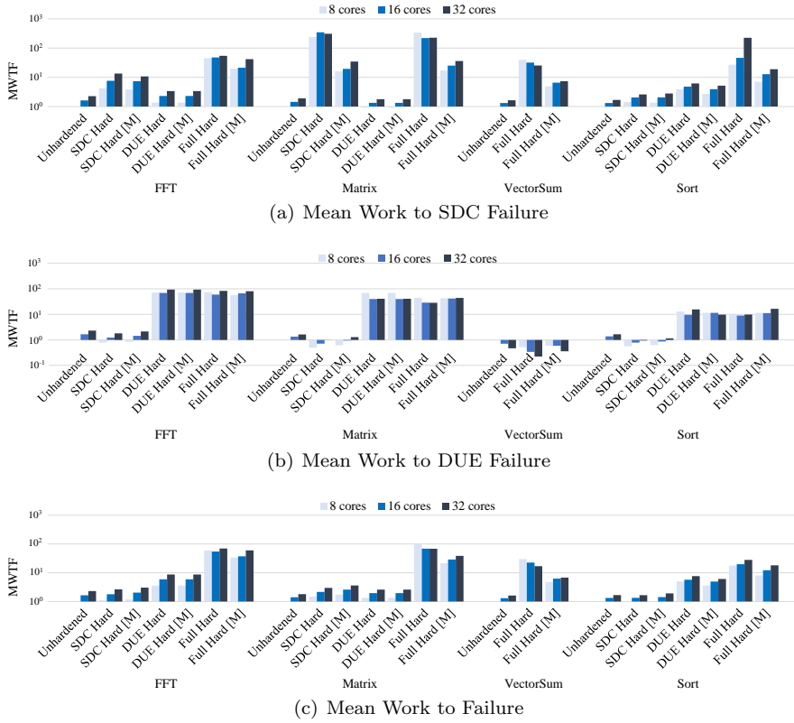
Fig. 7 MWTF normalized over original 8-core configuration. (a) Mean Work to SDC Failure. (b) Mean Work to DUE Failure. (c) Mean Work to Failure.
