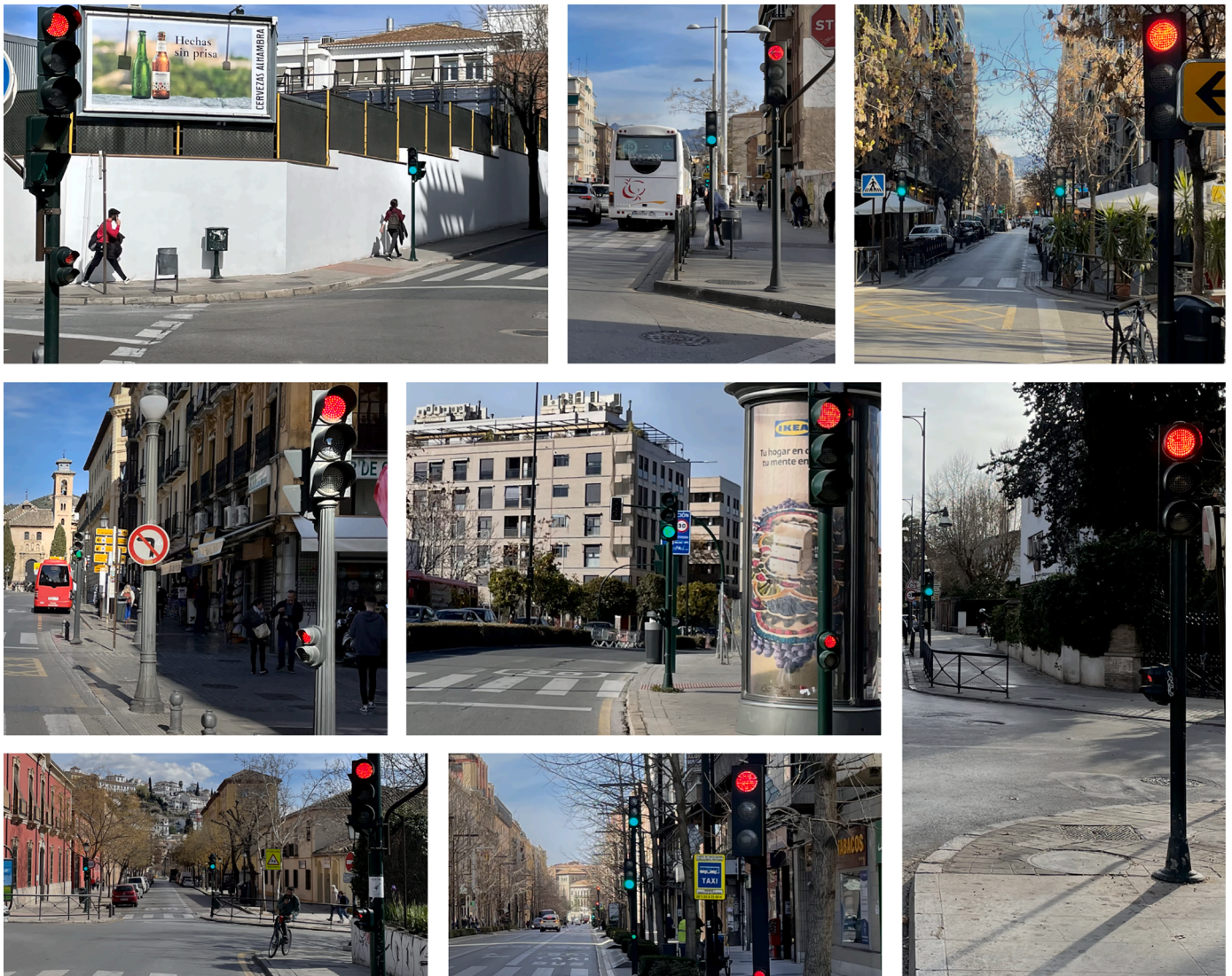
Fig. 1. Examples of competing sources of information at intersections in Granada (Spain): Short spacing between traffic light signals (range: 12 – 26 meters) displaying incongruent steady red-green lighting.
