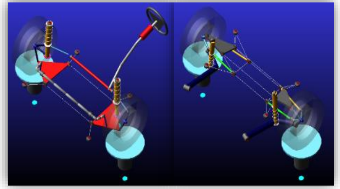
FIGURE 2 Front (MacPherson) and rear (multilink) suspension
