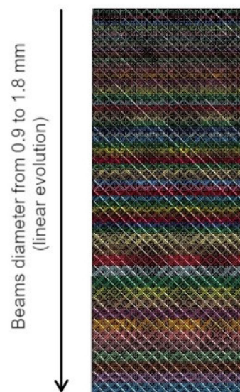
Figure 13. Geometry of the lattice crash absorber: linear variation of the beams' diameter.
