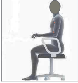
Figure 2 Seated dummy of typical tested subjects is shown. The two red circles represent bipolar connection of the upper arm with the ARMsense equipment.
