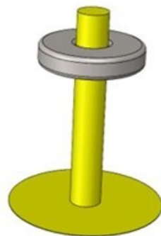
Figure 1. WEC mass properties, RM3 1:1 scale illustration [36].
