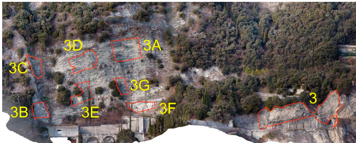
Figure 5. Rock face and survey windows (red polygons) analyzed in detail with non-contact surveys.
