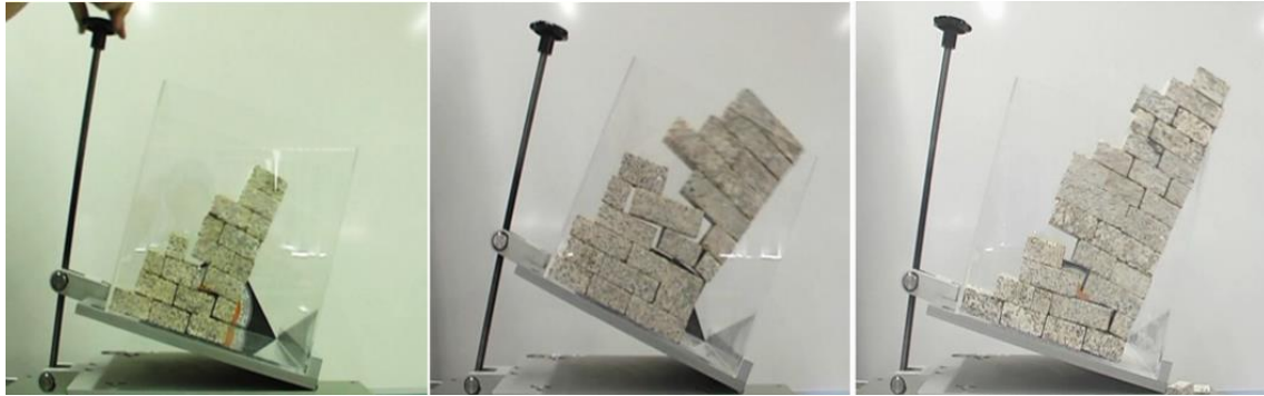
141 Fig. 2. Physical models of dry masonry retaining walls used to understand the failure mechanism 142 of these structures and check limit equilibrium calculations.
