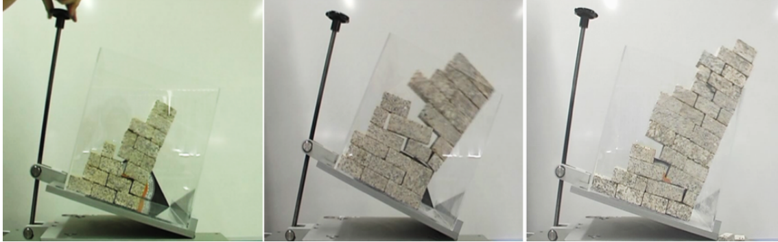
140 Fig. 2. Physical models of dry masonry retaining walls used to understand the failure mechanism 141 of these structures and check limit equilibrium calculations.
