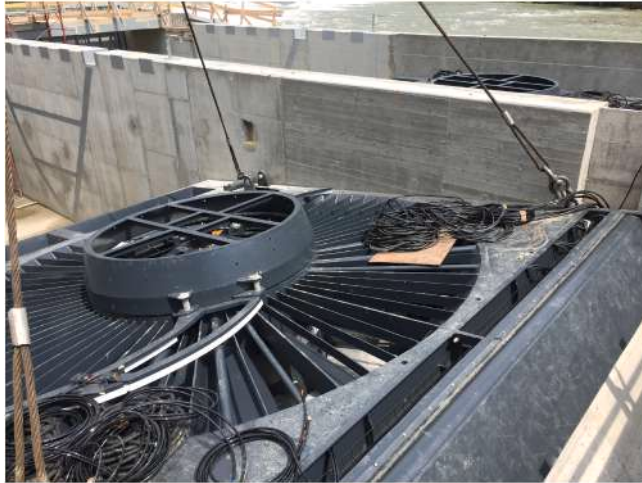
Fig. 4. Focus on the rack of the VLHT (Mazzè, Italy), photo Courtesy Geasiste.
