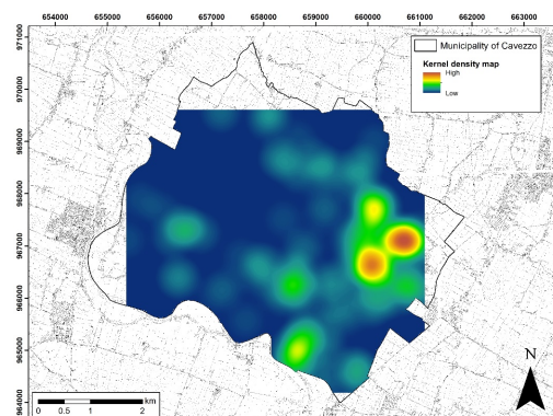
Figure 12. Kernel density map of the geotechnical investigation used to create the 3D engineering geological model of Cavezzo. The extension of the map is limited to the distribution of the available points.
