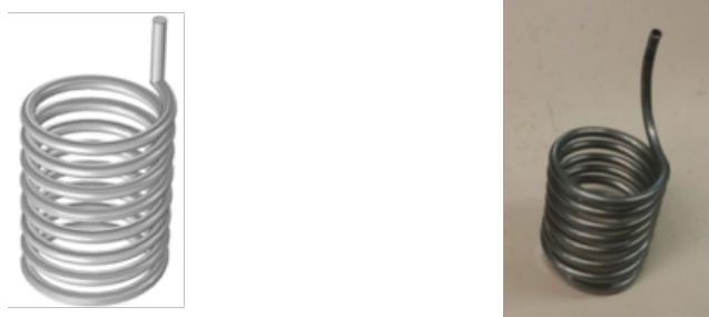
Figure 9: Helical sensor (drawing on the left, real helix on the right).
