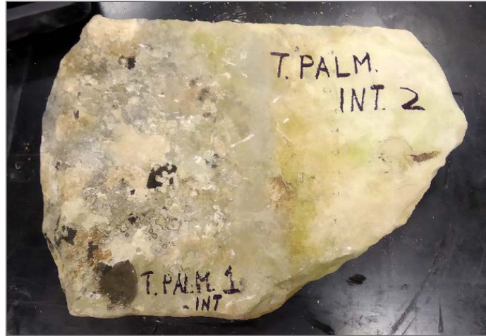
Figure 9: One half of this stone from Trullo Palmullo (in this case a chiancarella and not a sawn stone) shows evident signs of superficial weathering, which may be linked to mechanical properties. In this figure, taken before cutting, T. PALM. INT.1 refers to the TPI A side, whereas T. PALM. INT. 2 refers to the TPI B side.
