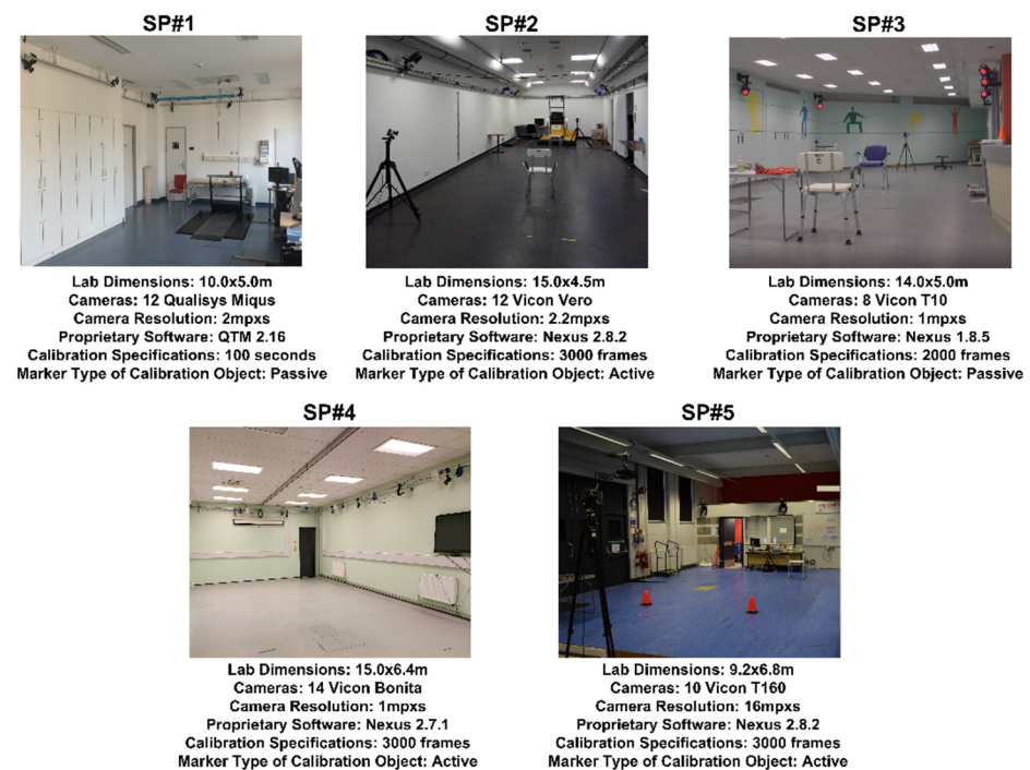
Figure 3. Specifications of each of the five SP systems (SP1–SP5) used in the multicentric deployment.
