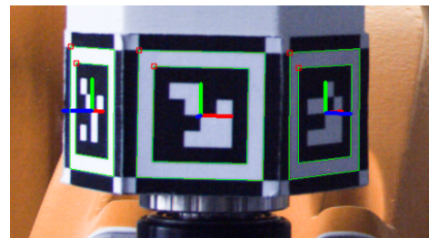
Fig. 1. 6DoF pose estimation of a robot endeffector with ArUcoE
